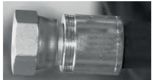
F) The shoulder of the stem should make contact with ferrule, if you install an elbow make sure the angle is right.
